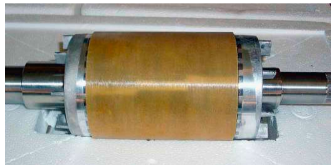
Figure 3: PM rotor complete, with bandage
