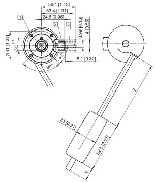
Insertion depth for blind hollow shaft 14.5 [0.57]
