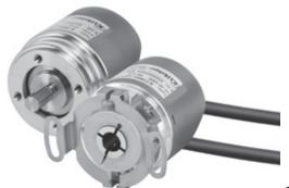
The Sendix F36 multiturn with the patented Intelligent Scan Technology™ is an optical multiturn encoder in miniature format, without gears and with 100% insensitivity to magnetic fields. With a size of just 36 x 42 mm it offers a shaft or a blind hollow shaft of up to 10 mm.
